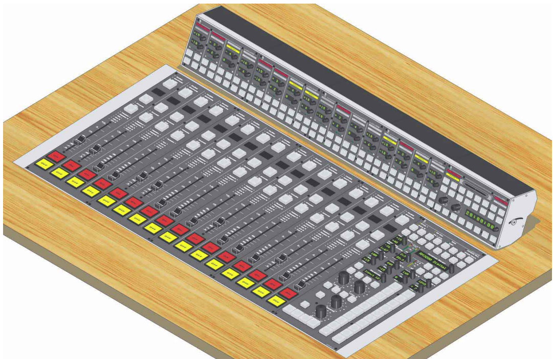
Figure 2: RM3200D Control Desk with new overbridge modules
