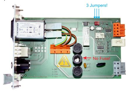
The Z420-845 Mains Power Inlet Module may be modified to become a Z420-845SLAVE by adding the 3 Jumpers and removing Fuse F1 (middle) to position F3 (upper).
