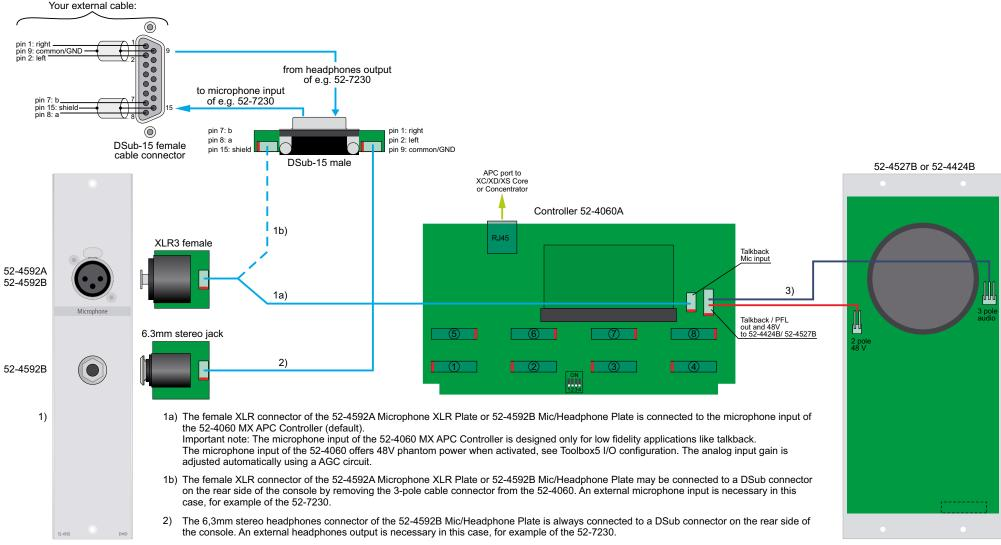
3) The loudspeaker amplifier of the 52-4527B or 52-4424B is connected to the analog output of the 52-4060 using a 5-pole cable. This 5-pole cable supplies also the 48V for the amplifier of the 52-4527B or 52-4424B.
