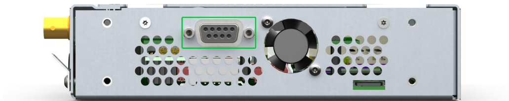
52-7420/52-7410 XC2 Core - side view with one male DSub-9 serial RS232 port
