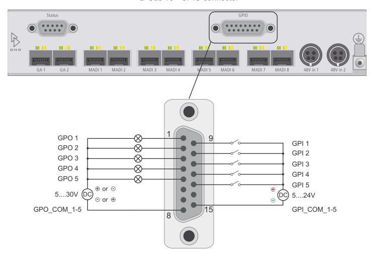
GPI - general purpose input GPO - general purpose output
