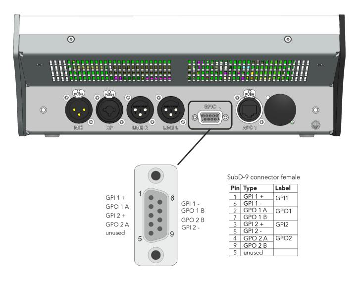
GPI - general purpose input GPO - general purpose output
