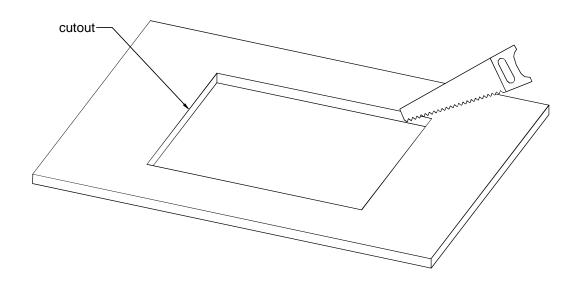
Cutout for Console Frame of Mixing Console 52/MX. For dimensions of Console Frame, see next page!
