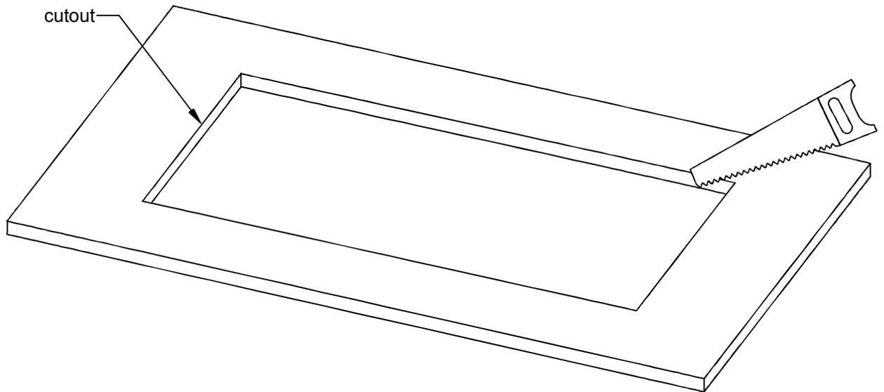
Cutout for Console Frame of Mixing Console 52/MX.
