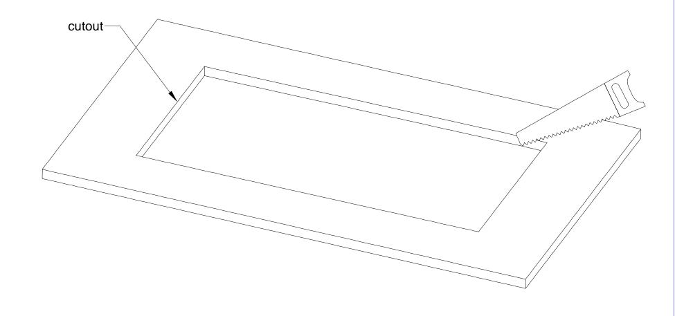
Cutout for Console Frame of Mixing Console 52/MX. For dimensions of Console Frame, see next page!
