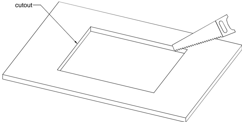
Cutout for Console Frame of Mixing Console 52/MX.
