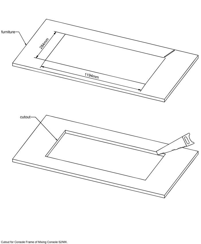
Cutout for Console Frame of Mixing Console 52/MX. For dimensions of Console Frame, see next page!
