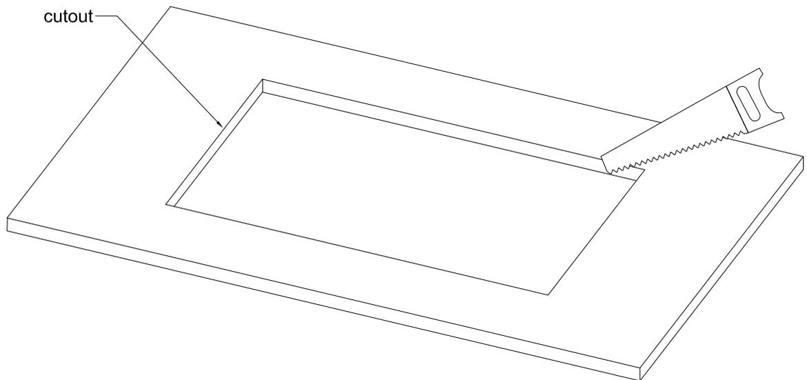
Cutout for Console Frame of Mixing Console 52/MX.
