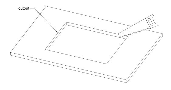
Cutout for Console Frame of Mixing Console 52/MX. For dimensions of Console Frame, see next page!
