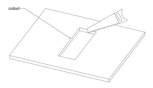
Cutout for Console Frame of Mixing Console 52/MX. For dimensions of Console Frame, see next page!
