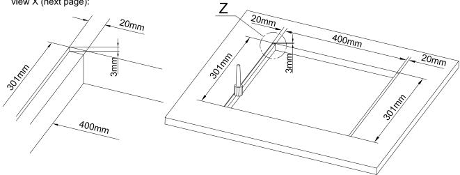
Cutout for Table-Installation Frame of Mixing Console 52/MX. For dimensions of Table-Installation Frame, see next page!
