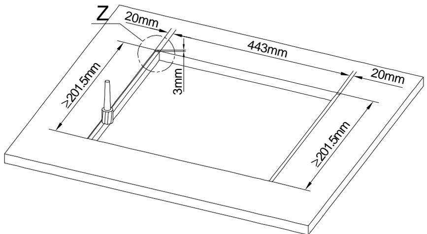
Cutout for Table-Installation Frame of Mixing Console 52/MX.
