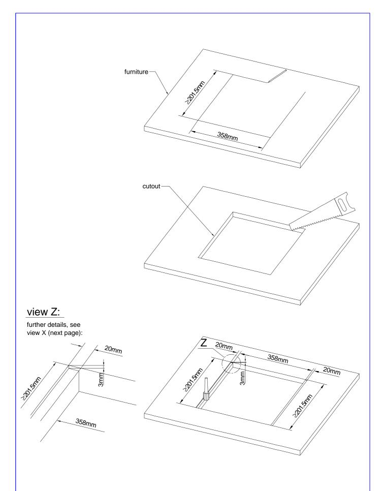
Cutout for Table-Installation Frame of Mixing Console 52/MX. For dimensions of Table-Installation Frame, see next page!
