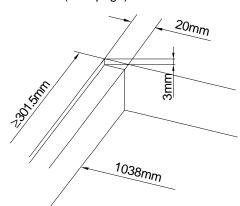
Cutout for Table-Installation Frame of Mixing Console 52/MX. For dimensions of Table-Installation Frame, see next page!
