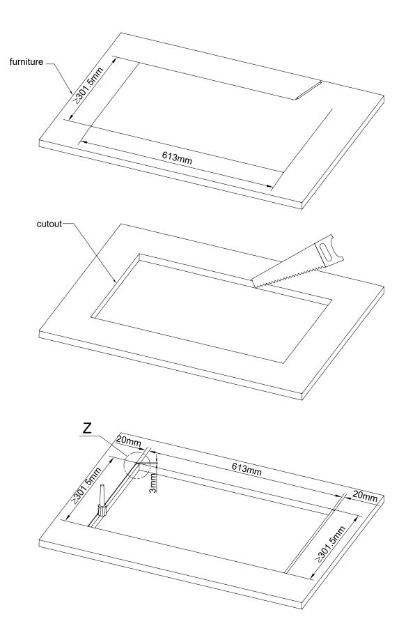
Cutout for Table-Installation Frame of Mixing Console 52/MX. For dimensions of Table-Installation Frame, see next page!
