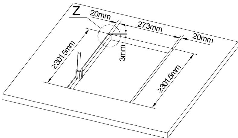
Cutout for Table-Installation Frame of Mixing Console 52/MX.
