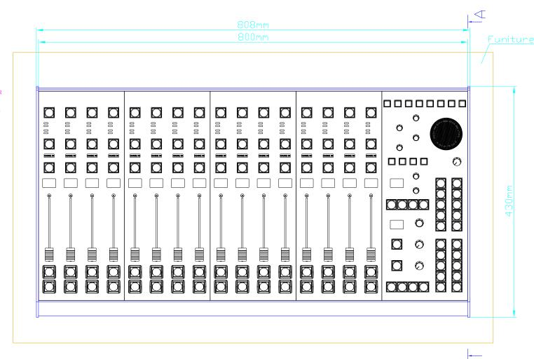
Console Frame for example Mixing Console 52/RX
