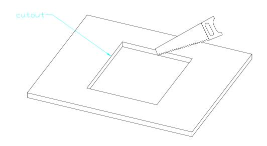
Cutout for Console Frame 52-2810 of Mixing Console 52/SX. For dimensions of Console Frame, see next page!
