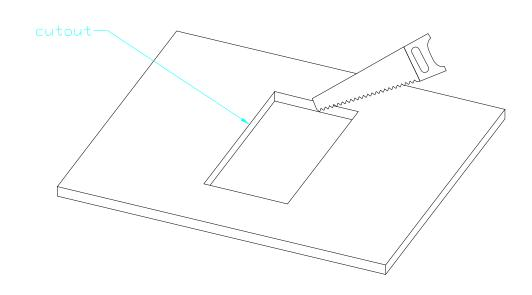
Cutout for Console Frame 52-2806 of Mixing Console 52/SX. For dimensions of Console Frame, see next page!
