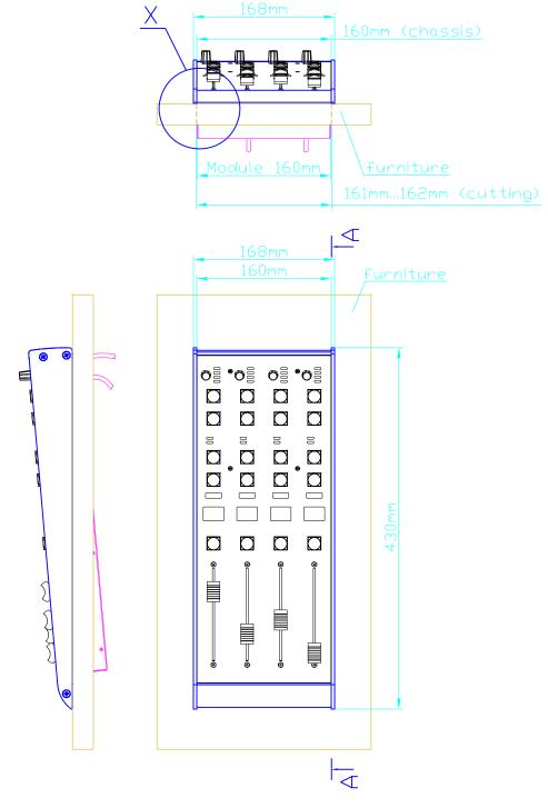
Console Frame for example Mixing Console 52/SX
