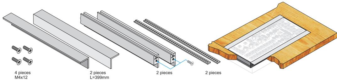
Figure 1-70: Example Table-Installation Frame
