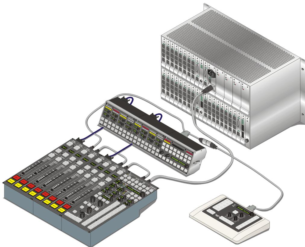
**Figure 1-1: DSP-Frame, Control Desk and Studio Panel coupled via CAN-Bus.**
