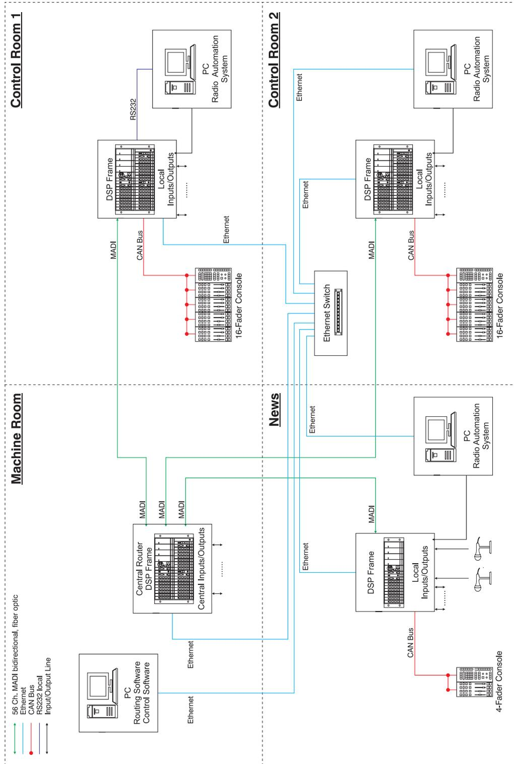
Figure 1-8: Central Matrix linked to three Control Rooms.
