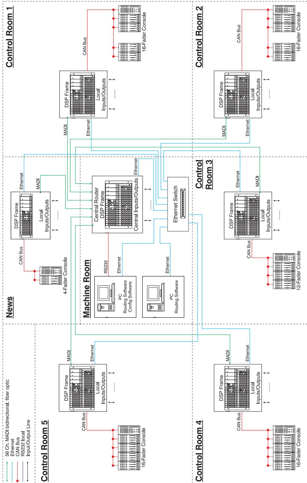
Figure 1-9: Large routing network application.
