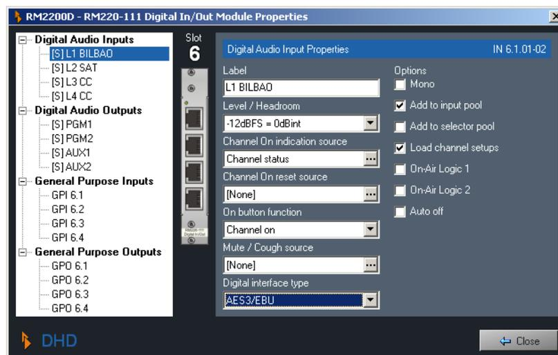
**Figure I-20: Configuration dialog for the RM220-111 Digital In/Out/GPIO module.**
