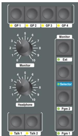
Figure I-7: Bottom part of the Master Control Module: general purpose keys, monitor keys, monitor potentiometer and talkback keys.
