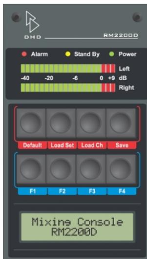
**Figure I-5: Top part of the Master Control Module: status LEDs, level meters, setup keys, function keys and the LC display.**
